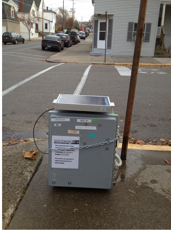
Figure 2: Continuous conductivity analyzer (typical).
